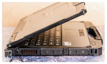
The covers can be slid into a locked position to ensure they stay closed, and rubber bladders on their insides create a tight seal to keep unwanted elements out.
