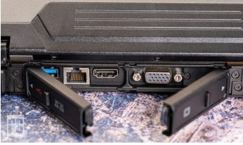
There's also a blank area next to the VGA port for another connection, and you can opt to outfit the B360 with a DisplayPort or USB Type-C port instead of the VGA port.
