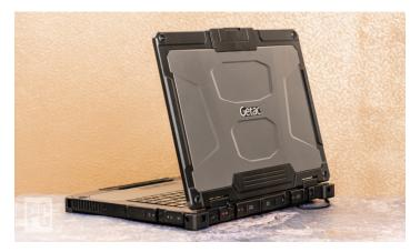
The molded top lid and built-in carrying handle are your first clues that the B360 is not an ordinary laptop but a rugged unit built for battle. At 5.1 pounds, the Getac is heavy for a 13.3inch laptop, but the extendable handle makes lugging the system easy and more secure than holding its edge. And the handle can be quickly snapped back into place so it doesn't interfere with your typing.
