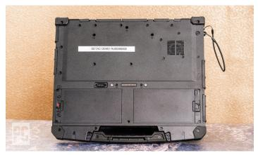
On the bottom panel are two user-removable batteries, which can be hot-swapped to keep mission-critical tasks on schedule without retreating to a wall outlet.
